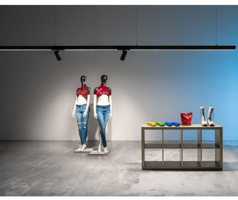
Combining lighting solutions with TECTON keeps them flexible in the long term. Luminaires that already installed can be moved easily, and additional luminaires can simply be clicked into place where desired.
